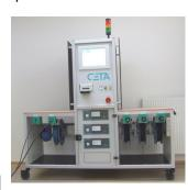
tolerances and the circuits must be leakproof. A special mobile multi-channel testing system, specially developed for this application, allows to perform pressuremonitoring and leaktesting on several hundred vehicles a day within the manu-
