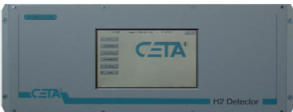
lows to detect leak rates up to  $1 \times 10^{-5}$  mbar\*l/s (corresponding to  $6 \times 10^{-4}$  ml/min). The device measures the quantity of gas escaping (concentration), which is proportional to the size
