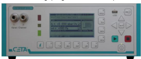
ther with channel 1, channel 2 or both channels. The function „endless filling“, which can be activated for each channel independently, supports the search for leaks in the adaption. On the front, there are two test leak connections as well as the USB connection for storage media. These can be used to store measuring series, curves and
