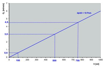
Leak-tightness of a product should be defined by the **leak rate.**
