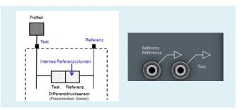
However, if a master part is connected and a test leak is also connected to the test leak connection of the test device, unexpectedly high pressure loss values are measured (the test leak is only connected to the internal measuring circuit volume (a few cm<sup>3</sup>), but not to the master part).
