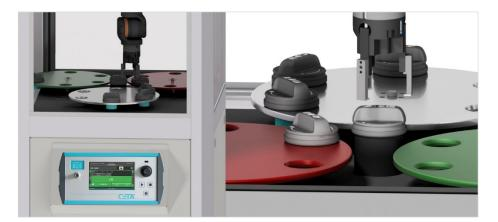
Test stand for leak testing of fuel tank caps - *Left:* Detail of test cell with leak tester and robot handling *Right:* Detailed view of the adaptation with inserted fuel tank cap and product holders in rotary tables\*
